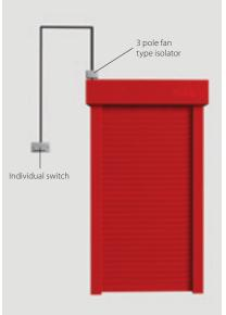
Control mechanisms are available as both single motor and group command activated motors for multiple shutters, so that shutters can be operated individually or in groups. Single rooms can be controlled individually, ensuring that the shutters are only operated in full sight of the user.
