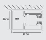
The guide rail is manufactured from extruded aluminium with a box section for fixing and high density 5 mm pile brush seals. The H34 guide profile is supplied as standard. The rail must be rebated behind the outer brickwork to achieve maximum security.
